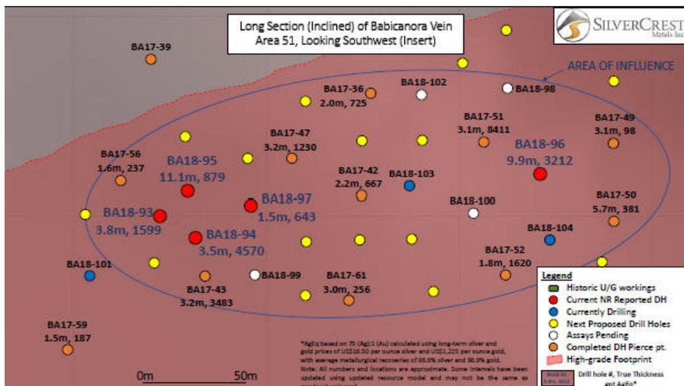
Figure 2: Long Section (Inclined) of Babicanora Vein Area 51, Looking Southwest
